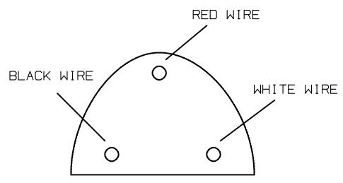
FEMALE CONNECTOR AT END OF SPEEDOMETER CABLE THAT PLUGS INTO THE HALL EFFECT SENSOR ON THE REAR WHEEL DROPOUT.
