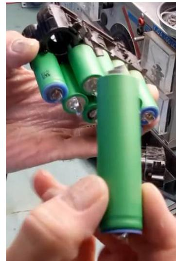
7. LAST STEP... FOLD COMPLETELY THE TABS ONE ON THE OTHER WHICH WILL BECOME THE SOLDERING CONTACTS FOR THE CIRCUIT CONFIGURATION YOU CHOOSE AS DESIRED. (YOU CAN USED THE BACK OF THE SIDE CUTTER TO GENTLY SMOOTH THE TABS)
