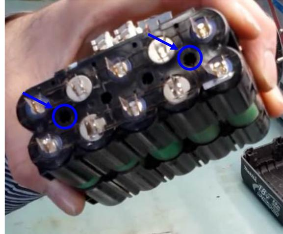
6. REMOVE THE BMS... EITHER WITH THE SIDE CUTTER OR PRYING UNDER THE ELECTRONIC BOARD WITH A FLAT SCREW DRIVER.
