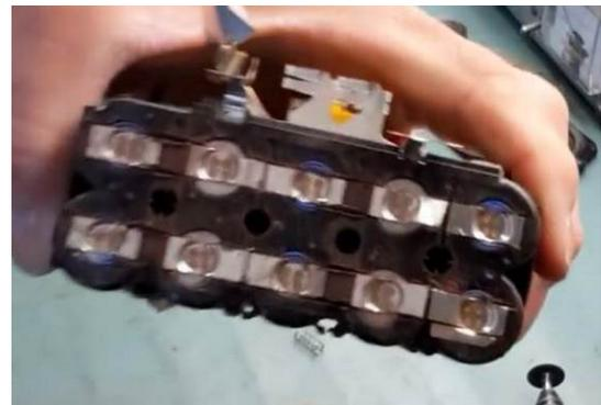
5. YOU WILL NOW (TEMPORARELY) FOLD THE REMAINING TABS AT 90° TO ALLOW YOU TO REMOVE THE CELLS FROM THE CASE... THERE ARE ALSO 2 TORX SCREWS TO BE REMOVED TO SPLIT THE CASING IN HALF.
