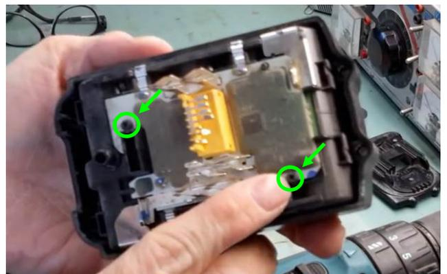
3. THE BATTERIES NEED TO BE SEPARATED FROM THE BMS (ELECTRONIC CIRCUIT) AND THE CASE... THE NICKLE PLATE (TOP AND BOTTOM) MUST BE CUT WITH THE DREMEL... ACCORDING TO THE PATTERN SHOWN BELOW...
